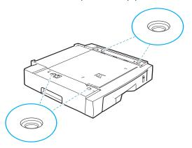
4 Place the machine over the tray, aligning the feet on the machine with the positioners of the tray.
